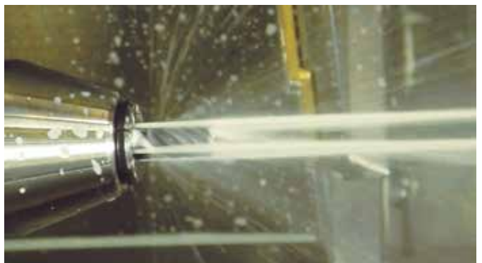
Using Reduction sleeve HS-CF - for peripheral cooling.
